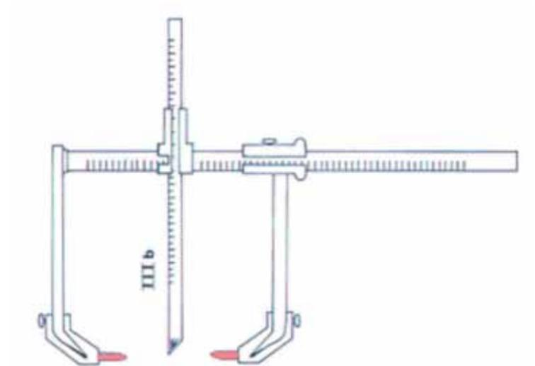
**Figure 9.** This is a radiometer (coordinate caliper) used for taking radii. The radiometer point is simulating the placement of the probes (in red) in the EAMs. Notice they are parallel and would “float” in the EAMs (Image from: Howells 1973, p. 164).
