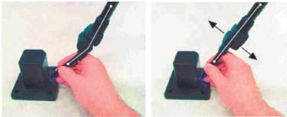
**Figure 3.** The image on the left demonstrates the correct way to take a bound point with the joint bent intentionally. The image on the right shows the incorrect way to take a bound point in which the stylus and forearm are aligned (Revware Systems 2009).
