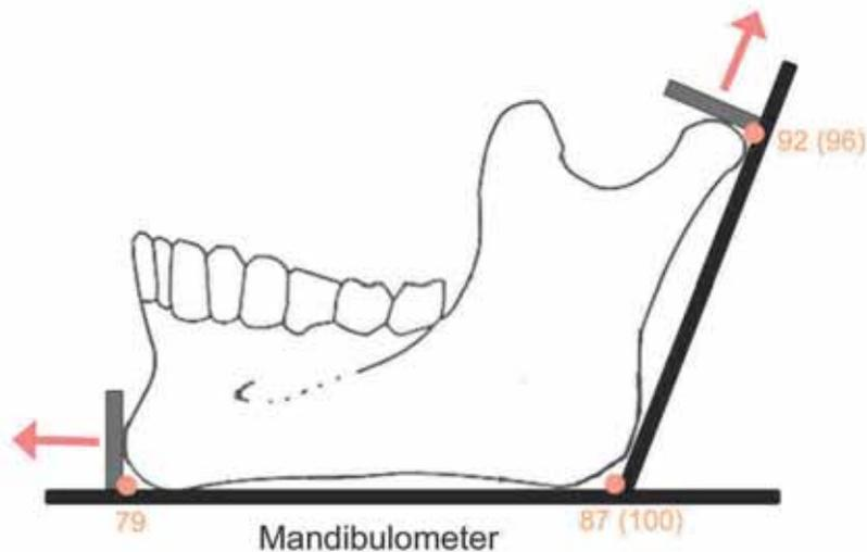
**Note:** After the mandible is positioned in the mandibulometer, pull back the horizontal and vertical sliding plates (arrows) so the digitizer stylus can reach the horizontal and vertical boards of the mandibulometer to capture the points.
