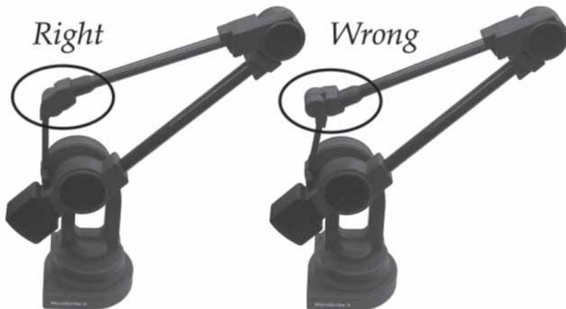
**Figure 1.** Correct and incorrect resting position (AKA Homing position) (Revware Systems 2009, MicroScribe G User Guide).
