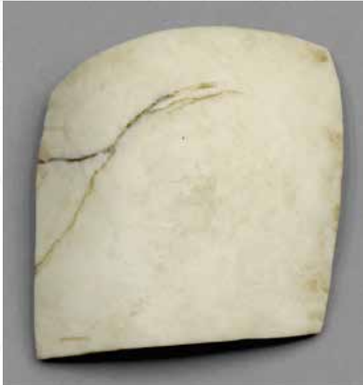
Fragment 5: Shearing Fracture Front View
