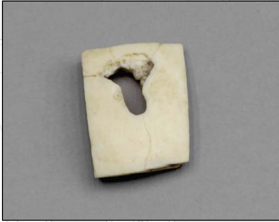
Fragment 1: Bursting Fracture Front View
