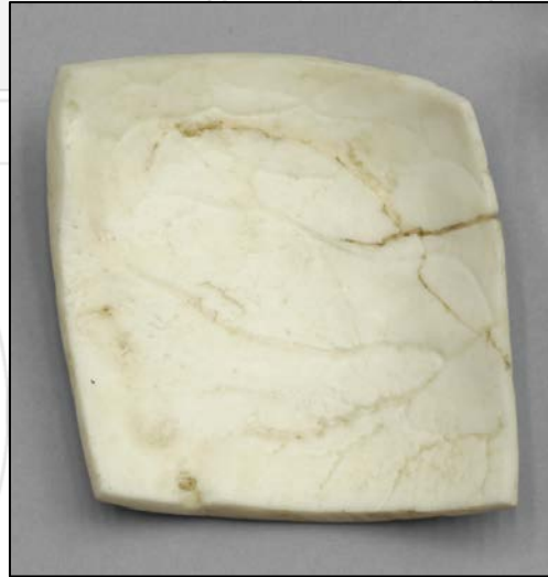
Fragment 5: Shearing Fracture Back View
