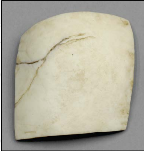
Fragment 5: Shearing Fracture Front View
